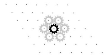
Under normal utilization, when the tractor is started, some of the gears are initially activated and try to turn clockwise. When a gear tries to turn in one direction, all the adjacent gears try to turn in the opposite direction.
