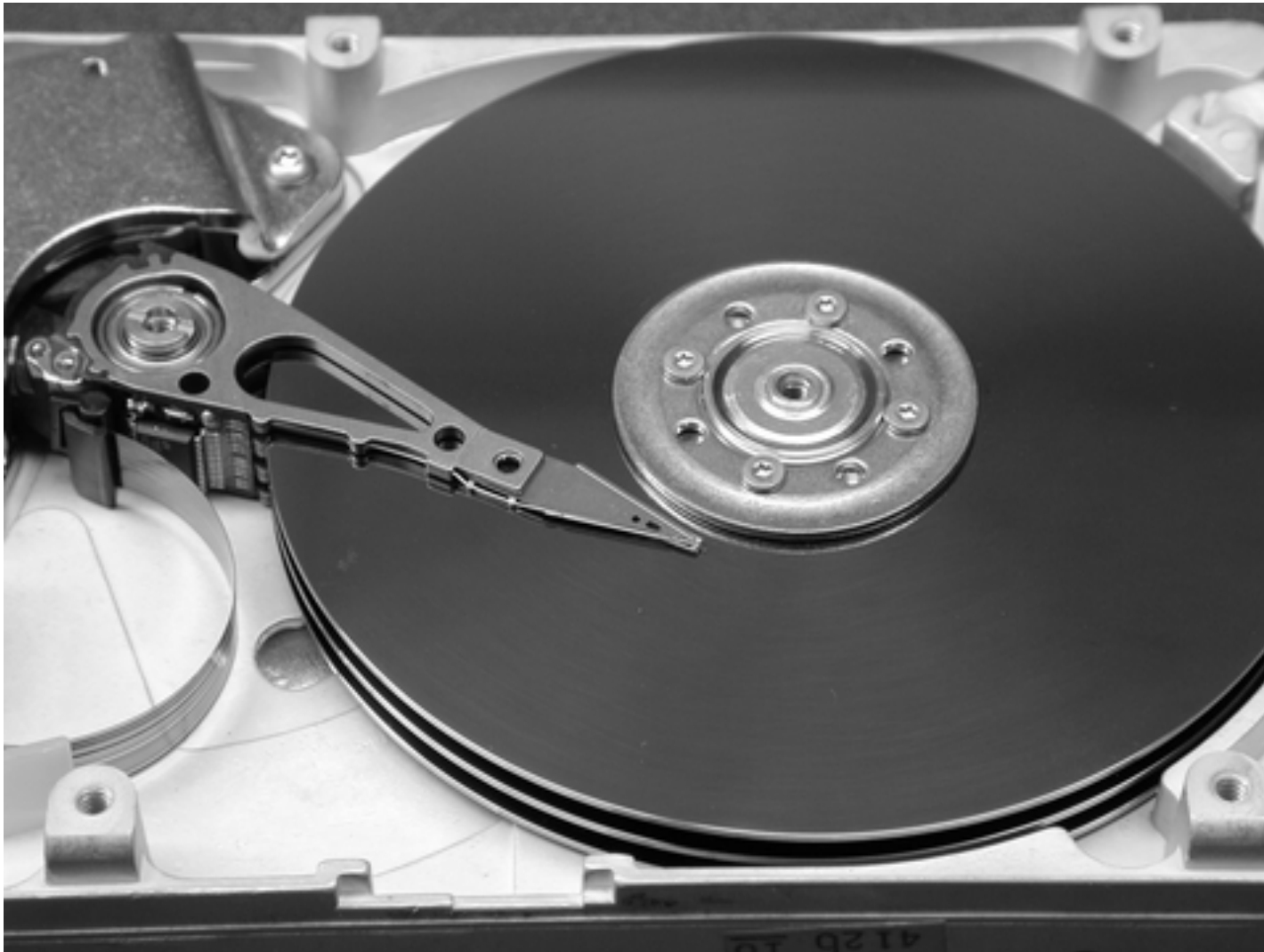
Steadily rotating platters and read/write heads of a HDD
