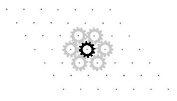
Under normal utilization, when the tractor is started, some of the gears are initially activated and try to turn clockwise. When a gear tries to turn in one direction, all the adjacent gears try to turn in the opposite direction.
